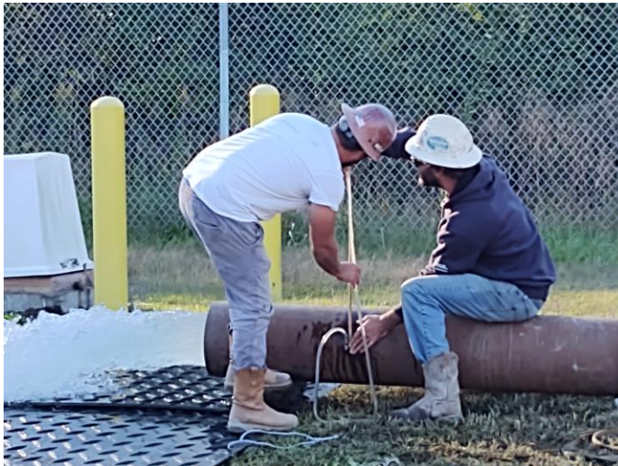
NP_MAR_01 pumping 2,800 gpm during testing
