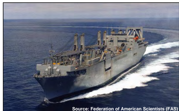
T-AKR 295 Shughart is a Large, Medium-speed, Roll-on/Roll-off Ship (LMSR) converted from the ex-Laura Maersk commercial vessel.
