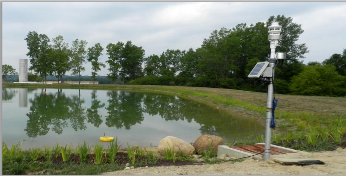
Figure 4: Continuous Monitoring and Adaptive Control Station Implemented at a Wet Pond
